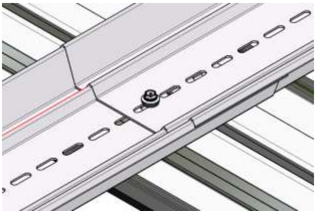
Figure 56 Overlap the ballast rail and mount it with a Self-Drilling-Screw 4.8x19
