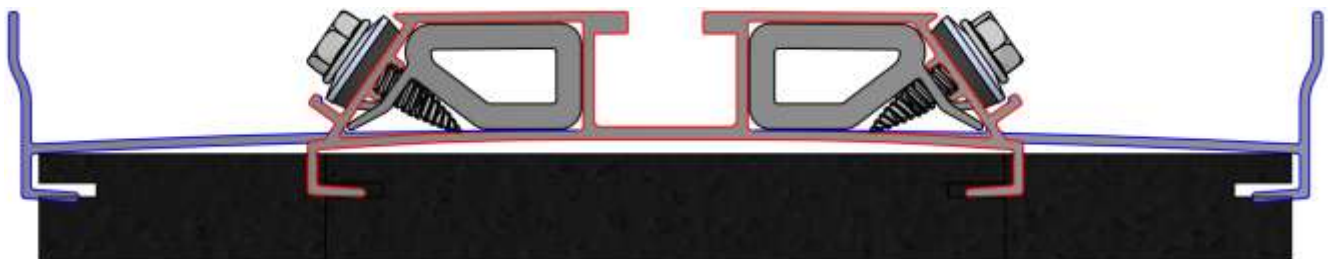
Figure 20 Section view base rail G3 (blue) and G3 Eco (red) with internal butt connector
