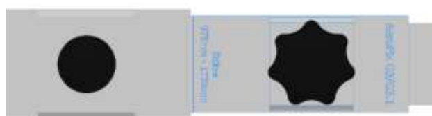
Figure 34 Set the middle tube of the jig on the side at “AeroFix G3 /3.1” to the locking point “Support 975 mm - 1730 mm.”
