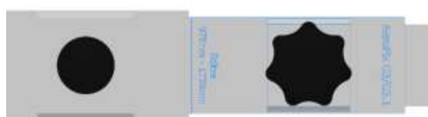
Figure 50 Set the middle tube of the jig on the side at “AeroFix G3 /3.1” to the locking point “Support 975 mm - 1730 mm.”
