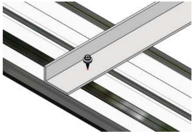
Figure 62 Place Alu-L-Profile on position and fix it with Self-Drilling-Screw 4.8x19 on the base rail.
