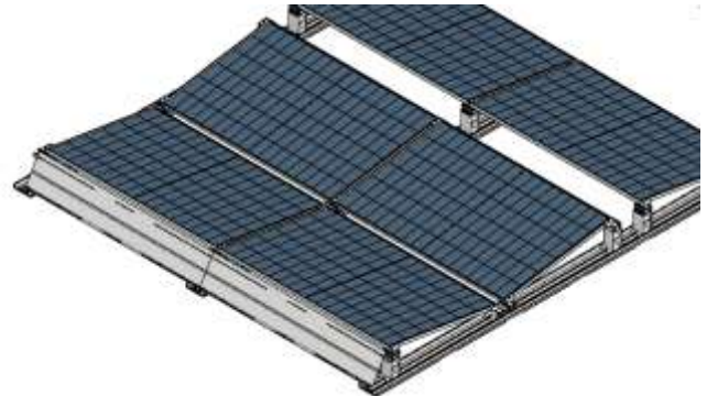
Figure 80 Mounted wind plates on the East-West systems
